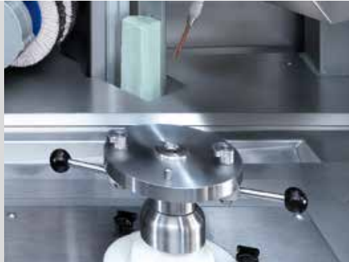
3-axis controlled cross- and rotary table
