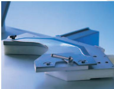
Cutter blade with straight cutting edges
